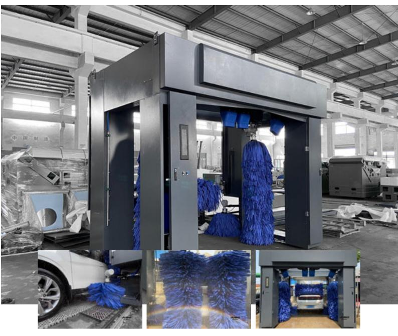
Fast, quiet, safe and reliable wash gantry - rollover car wash - JUBO JUBO wash gantry with standard 5 brushes spinning and cleaning the vehicle while the rollover gantry moving forward and backward, at highest speed 3 minute to wash a car, power0.1KWH and 60L water consumed.
